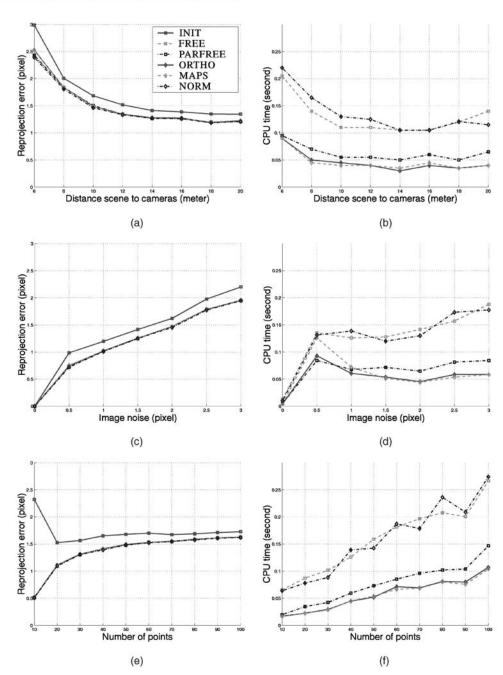
Fig. 1. Reprojection error (left column) and CPU time to convergence (right column) measured against different simulation parameters: distance scene to cameras (first row), image noise (second row), and number of points (third row). Concerning the reprojection error, the curves are almost always undistinguishable, apart from the initialization. For the CPU time, methods are divided into three groups: (from top to bottom) FREE and NORM, PARFREE, then MAPS and ORTHO.
