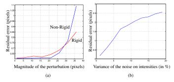
**Fig. 3**. Registration of simulated data. The results are median over 100 trials. (a) shows the residual error when the magnitude of the perturbation  $\delta_N$  or  $\delta_{NR}$  is varied. (b) shows the residual error for varying noise on the image intensities.
