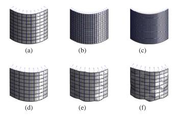
Figure 2. Test cylinders quantised into grids of (a)  $10 \times 10$ , (b)  $20 \times 20$  and (c)  $30 \times 30$  squared patterns. (d) Surface and normals recovered at short range ( $\bar{d}/f = 2.5$ ) with no noise. (e,f) Reconstructions with measurement noises (additive Gaussian with standard deviations  $\sigma = 0.1$  and  $\sigma = 0.2$ ) respectively
