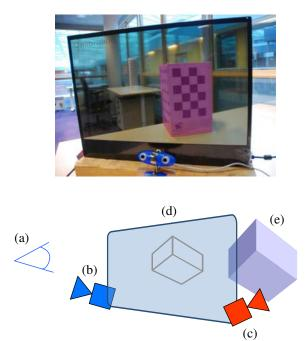
Figure 1: System setup. The components are: (a) user, (b) face tracking camera, (c) scene analyzing camera, (d) transparent screen, (e) scene
