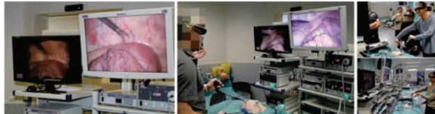
Fig. 1: Our current live monocular 3D laparoscopy prototype system. (Left): Two screens showing (white) the raw 2D video feed and (black) the reconstructed 3D with an active-shutter display. (Remaining images): System in use.
