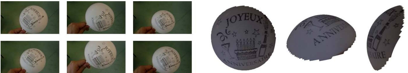
Figure 16: Experimental results using real conformal deformations – the balloon dataset, construction of the template. The left part shows some of the 8 images we used to reconstruct the 3D template shown on the right part with SfM.
