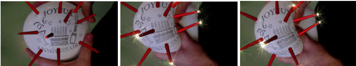
Figure 1.7: An AR SfT application from [Bar+15]. Video frames of a real deforming birthday balloon are augmented with 10 virtual candles. Using SfT, a balloon template is registered and reconstructed from each image. Virtual candles are placed on the template, and thanks to the registration and reconstruction provided by SfT, the candles can be automatically augmented on the images, giving the impression they are physically stuck to the surface and oriented appropriately. Furthermore, the candles can be virtually ignited when the balloon is squeezed sufficiently, thanks to the recovered 3D shape information.
