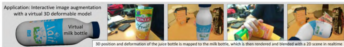
Figure 1.9: A Human Computer Interaction (HCI) SfT application from [CB15]. The goal is to assist a computer animator to interactively deform a virtual object by manipulating a real, similar deformable object in their hands. In this example the real object is a juice bottle that is viewed by a monocular camera. Its corresponding deformation and 3D position are recovered from the camera video with SfT. The deformations are transferred in real-time to a virtual object (a milk bottle). The deformed virtual object is then visualized for the animator. Using this setup, an animator can interactively position and deform the virtual object in a scene by physically deforming a real object. This may save them considerable time compared with standard deformation editing in graphics software.
