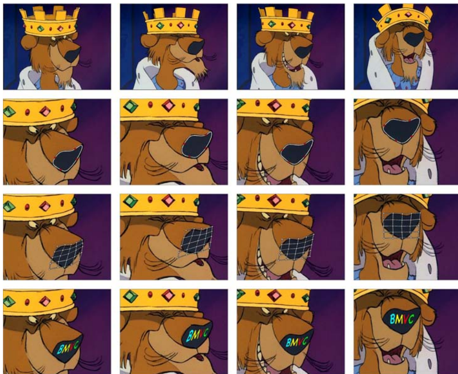
Figure 2: First row: 4 sample frames out of a sequence of 100. Second row: Corresponding curves with 4 points marked. Third row: Grid showing the deformations modeled by the TPS warp. Fourth row: The final retexturing.
