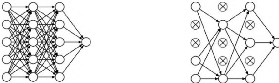
(a) A feedforward network with fully connected layers (used at inference). (b) The network after dropout (used in training). Neurons are randomly dropped at each epoch.
