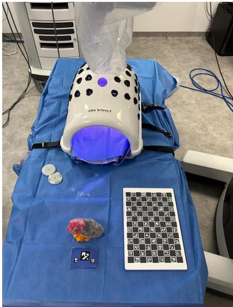
Figure 3: Experimental setup used for preclinical validation of the AR prototype. From top to bottom and left to right: Da Vinci stereoscopic endoscope, Pelvitainer box trainer, 3D-printed kidney model coated with AESUB spray, ArUco marker, and calibration checkerboard.
